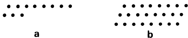
Figure 2 (a) An (8,3) equivalent group and (b) an (8 × 3) closed group, both shown in projection with the {110} direction horizontal
